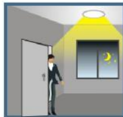
When motion is detected, the sensor brightens the lamp to 100% illumination.
