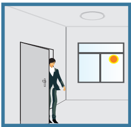
With sufficient ambient light, the sensor does not switch on the lamp.
