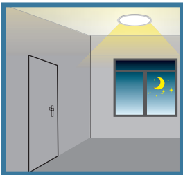
No motion detected, the lamp remains at a low light level all the time.
